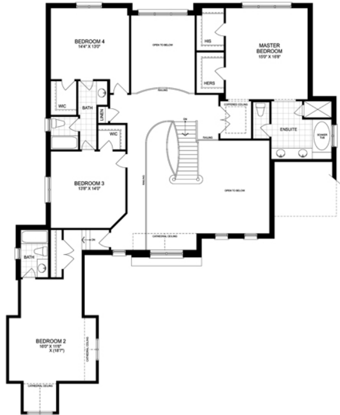
SECOND FLOOR ELEVATION 'A'
